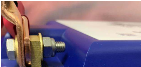
Proper Connection: Longer bolt used with multiple lugs can fully seat into nylon insert of nut without interfering with battery case
